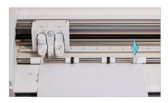
Lower the release lever. On the Cameo 3, twist the roller body to the unlocked position. Slide the roller over to the desired groove so it settles in place. Twist to lock the roller again. Pull the release lever up so it's pointing up and locks the bar in place.
