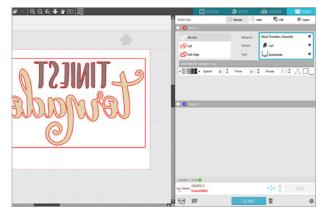
If you're using your heat transfer for the first time, you should make a test cut to verify the default settings work with that material. Move the design over toward the right so there's room for a test cut in the upper left corner.
