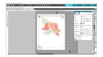
One thing to watch for in ready-made Print & Cut designs is the line thickness. You want the line thickness to be 0.0 so the cut line doesn't print.
