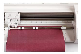
Any time you're cutting directly from a roll, you need to adjust the rollers on the Cameo so they grip the material securely on both sides.
