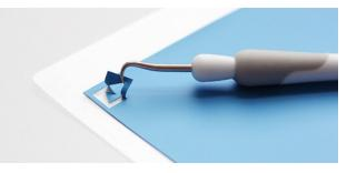
If the test cut is not coming cleanly off the liner, then adjust your Force or blade settings, use the on-screen arrow keys to move the blade to a new area on the mat, and make a test cut again.
