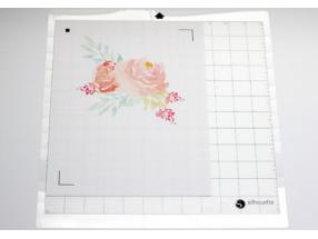
Click Send in the software. The Silhouette machine behaves the same way with any Print & Cut by finding the registration marks before cutting.
