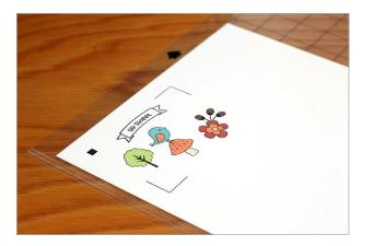
The machine will read the registration marks before cutting when you have registration marks turned on in the document.
