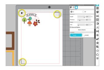
Those marks tell your machine where your cut lines are in relation to those marks, so it can compensate for things like the differences in how you load your media and mat each time. The crosshatch area is the area where you need to avoid placing your designs. As the machine moves to each registration mark, it shouldn't have anything in the crosshatch area because that could confuse the optical eye.
