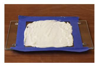
Do not scrape the cream or push hard against the glass; the cream could seep under the stencil's edges.
