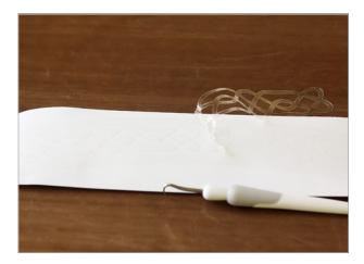
Use a piece of transfer tape large enough to cover the design and smooth it against the design with the scraper tool. Then pull the stencil and transfer tape all off the backing together.
