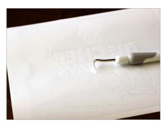
Use the hook tool to weed the vinyl, removing the outside edge first, where it touches the outer edge of the vinyl backing.
