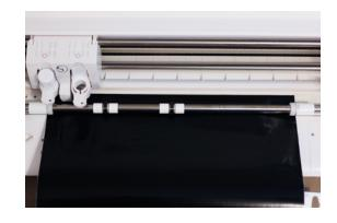
When the vinyl is loaded correctly, you should see the front edge appear straight all the way across and the rollers should be firmly gripping both sides of the vinyl.
