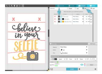
Make sure the Material for each color shows Vinyl, the Action shows Cut, and Tool shows AutoBlade or ratchet blade.
